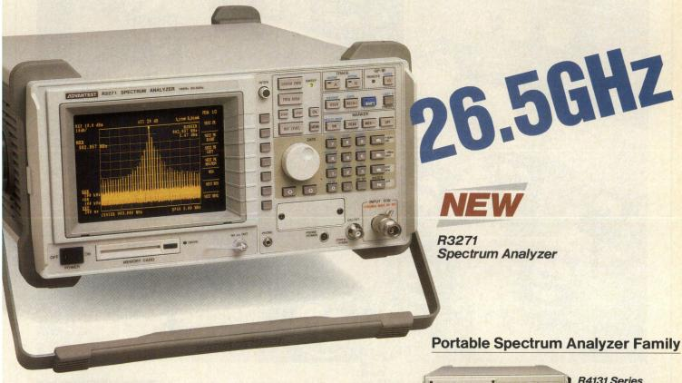
The Advantest R3271 Portable Spectrum Analyzer with wide 10Hz to 3MHz IF filter is capable of continuous repetitive sweep and measurements from 100Hz to 26.5GHz. An 8-point multi-marker and list display functions simplify spurious measurements and low-signal response measurement. The high-speed 5µs/div sweep and digital readout make it the optimum choice for mobile communications research and development.
