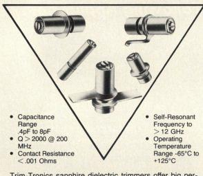
Trim-Tronics sapphire dielectric trimmers offer big performance in a small size with a variety of mounting styles. The rotor can be sealed to prevent intrusion by solder flux and/or cleaning solutions.
