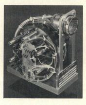
matched performance over a DC-20 GHz frequency range. Its compact size shortens signal paths and reduces insertion loss. Phase tracking is  $\pm 1$  degree at 1 GHz, increasing to  $\pm 5$  degrees at 20 GHz. Amplitude tracking is  $\pm 0.1$  dB to  $\pm 0.3$  dB over the same range. Minimum isolation in the 8-20 GHz range is 55 dB. The size of the unit is just  $5.5 \times 4.0 \times 5.0$  inches.
