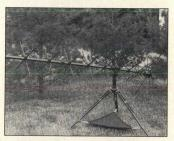
communications is announced by ADM. The ADM-C2 has right-hand circular polarization, with 10.25 to 14.4 dBic across the band. It will handle 200 watts, and includes a lightweight tripod for mounting.
