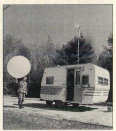
This radiosonde balloon uses a small, battery-powered telemetry transmitter to radio data to the ground station.
